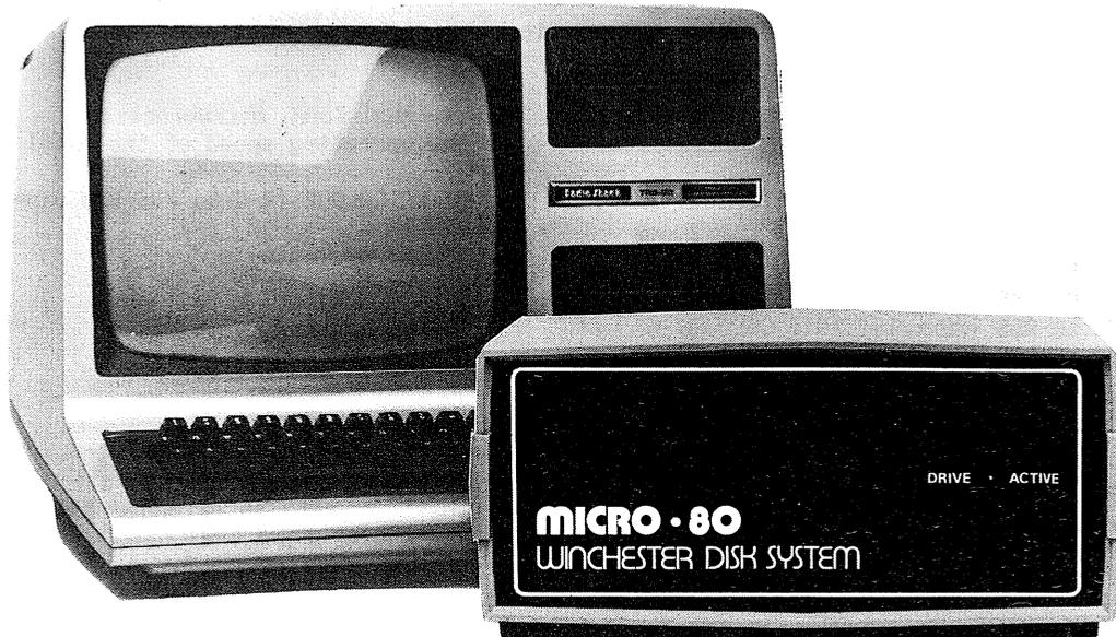
MICRO-80 fits reliable MPI disk drives to the TRS-80 Model 3 to give system capacities and capabilities far in excess of those available elsewhere. All our conversions utilise low dissipation, switching-mode power supplies to avoid screen jitter and overheating. The disk controller boards used incorporate special compensation circuitry for 80 track disk drives and may also be used to run 8 inch disk drives with an appropriate cable and DOS.
